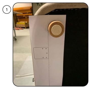
Cut a cross in the paper template for the legs and mount both legs over te template.
