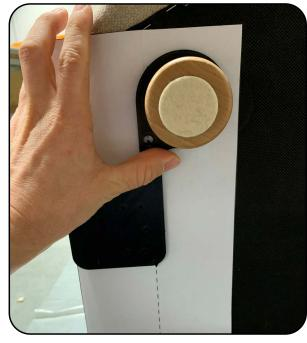
Place the drill template over the leg and make sure to point the arrow heads over the dotted line. Use the pilot holes in the template to drill through both templates.
